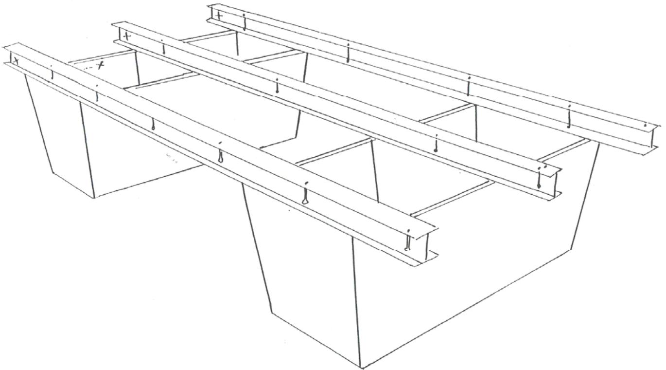
3. Place the bottom-frame on the steelbeams. The heatingssystem is integrated in the bottom-frame. **Please test the function of the heating parts before continuing the setup of the table.**
