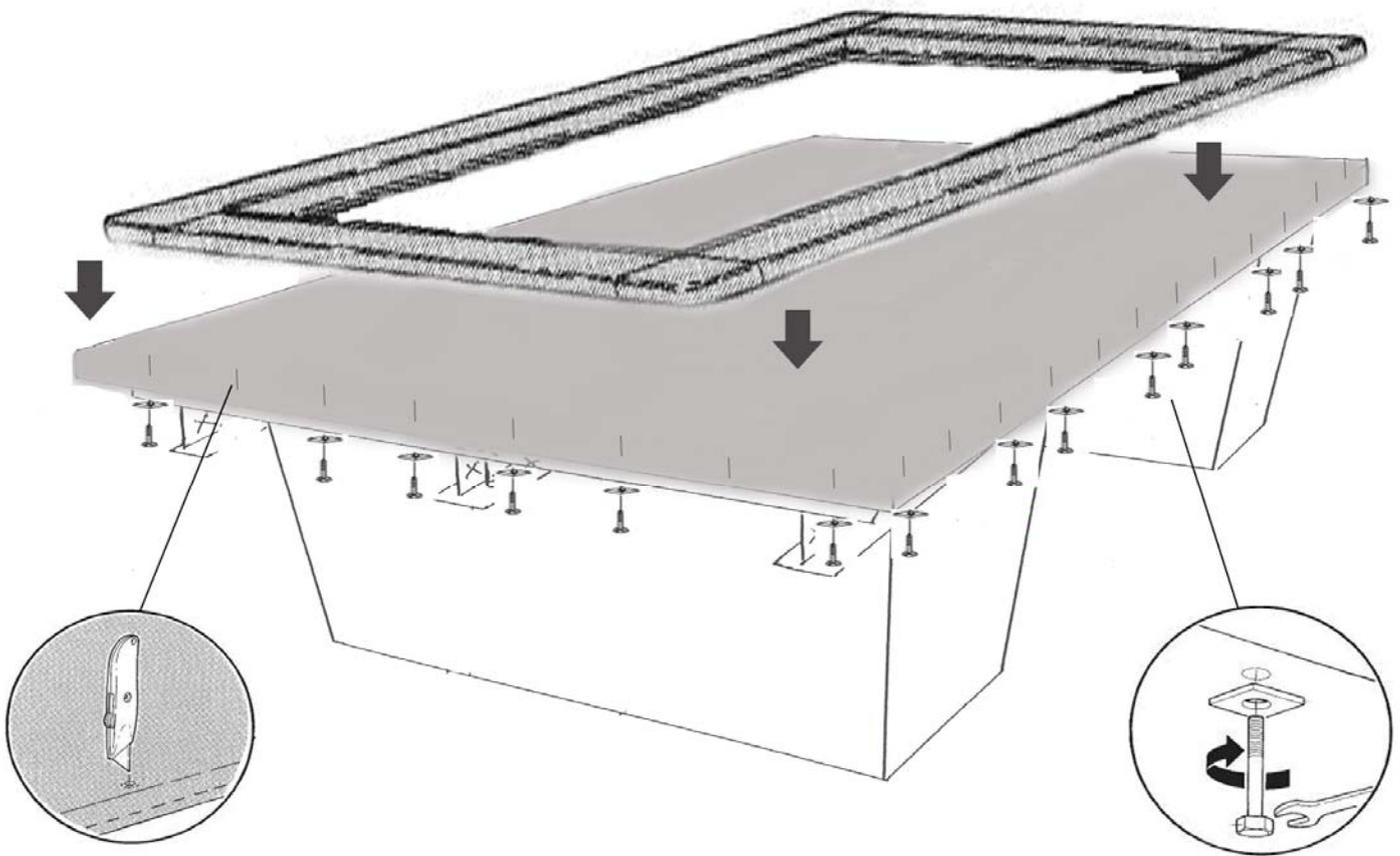
12. Last but not least – assemble the sides so they make a frame. Install the angle hinges to the sides with the screws. Finally put frame into the pre-drilled channel in the cushion-frame and fasten with the last 12 pcs. of loose **BLACK** bolts. Then fasten the bolts and your table is ready!
